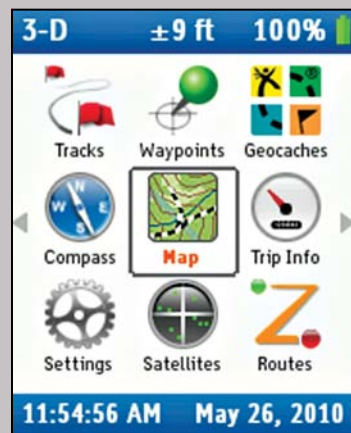
Home Page —Quickly choose the page to use, switch between pages, and view GPS fix and battery info.
